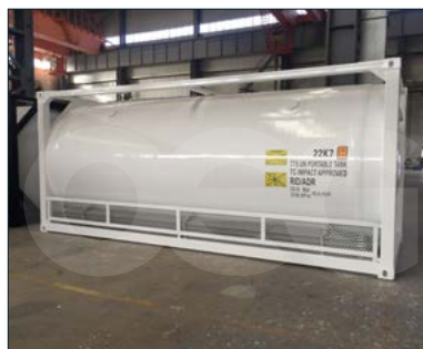
20ft Cryogenic Tank
