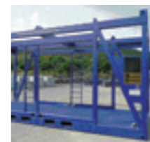
6.4m Lifting Frame Lifting Frame 6488 x 2838 x 3285 5660 19,340 25,000
