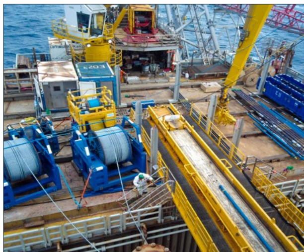
Spooling units simultaneously deploying ESP, Chemical Injection, Gauge and SV - Norwegian Continental Shelf (2021)
