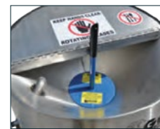
Push Rod Keeps Hands at a Safe Distance During Operation
